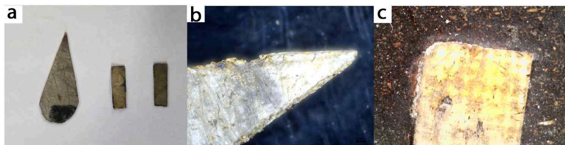
Fig. 9. Observation of tortoiseshell substitutes. (a) Detached specimens of the phoenix feather and Eight Trigrams (smartphone photographs), (b) microscopic observation of the detached phoenix feather (scale bar: 200 \mu\text{m} ), (c) microscopic observation of the detached Eight Trigrams specimen (scale bar: 200 \mu\text{m} ).
