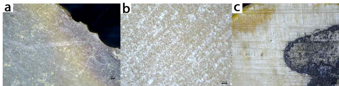
Fig. 10. Comparison of natural materials and the detached phoenix feather specimen. (a) Natural tortoiseshell (scale bar: 100 \mu\text{m} ), (b) ox horn (scale bar: 200 \mu\text{m} ), (c) detached phoenix feather specimen (scale bar: 200 \mu\text{m} ).
