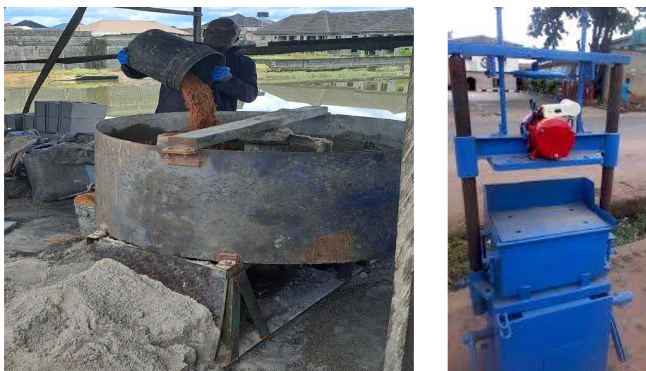
Fig. 4. Mixer and block semi-automated block moulder.
