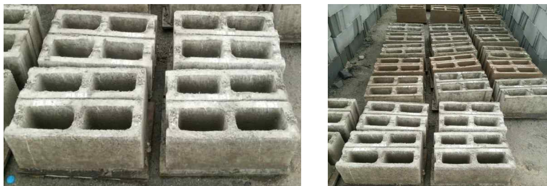
Fig. 3. Moulded blocks at different mix ratio.
