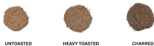
Fig. 1. Ground river red gum wood samples with different toasting levels.
