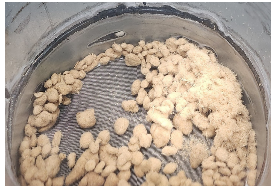
Fig. 8. Remaining wood fiber in drying tower.
