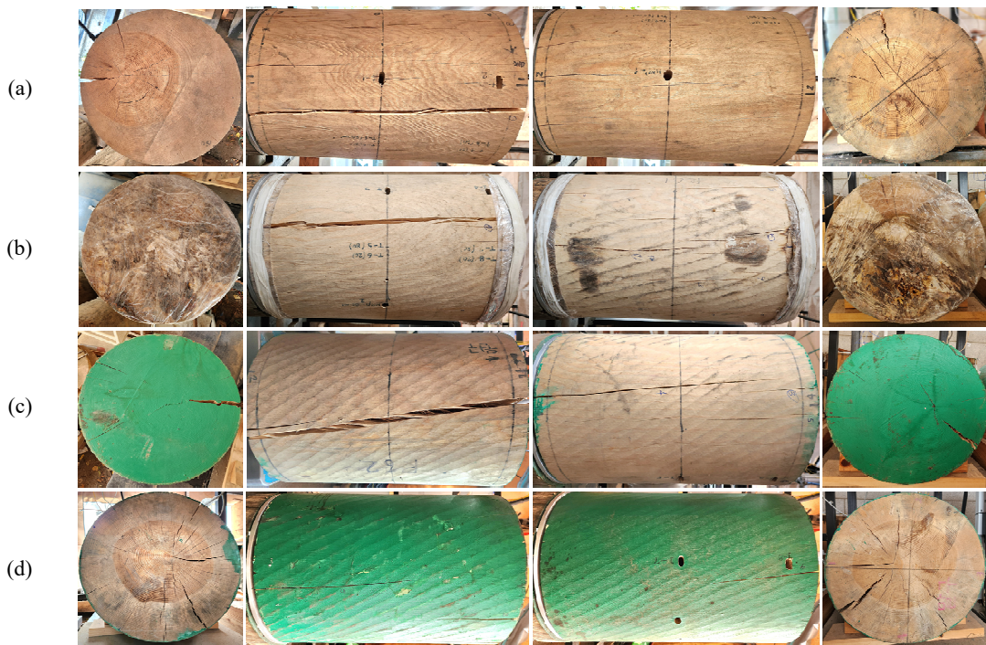
Fig. 10. Drying defects of large-cross-section timber. (a) Control; (b) end sealing; (c) end coating; (d) lateral coating.
