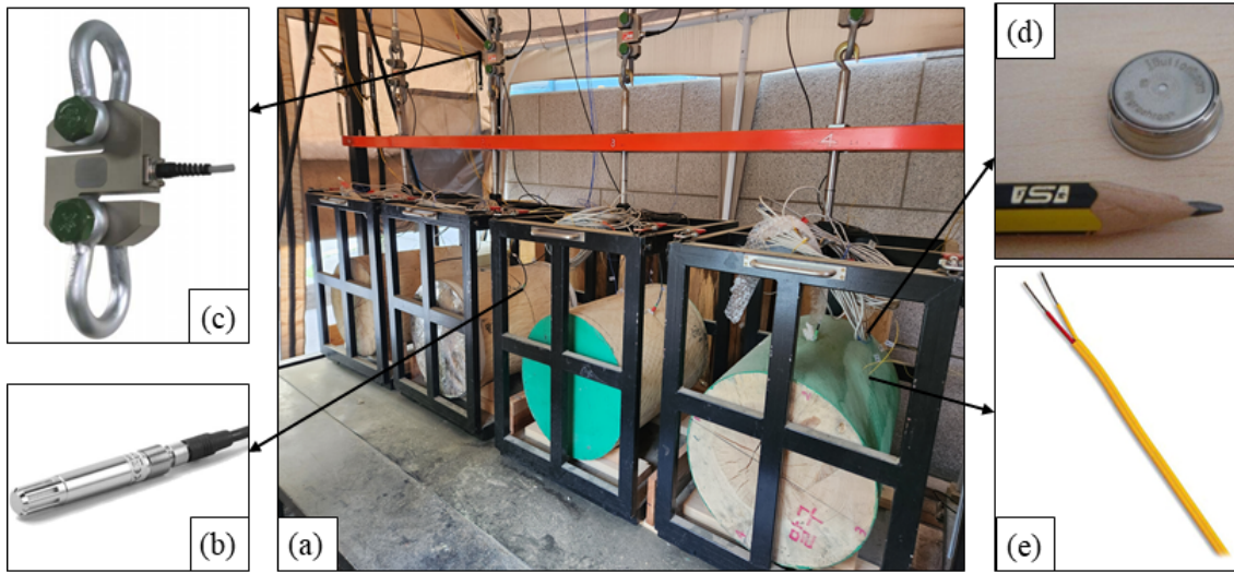
Fig. 2. Wood specimens mounted in a case with a load cell (a); VAISALA HMP60 humidity and temperature sensor (b); TLC-1t tension load cell (c); and iButton humidity and temperature sensor (d) and K-type thermocouples (e), inserted at multiple positions to measure the moisture and temperature gradient between the surface and core of the wood specimen.
