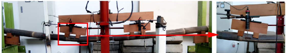
Fig. 16. Failure mode of Bamboo 2.
