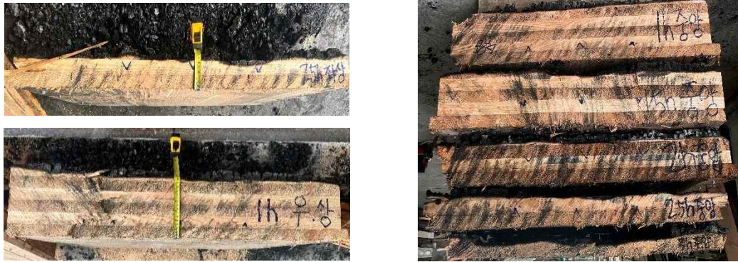
Fig. 4. Charring depth measurement and comparison of char depth by test piece.
