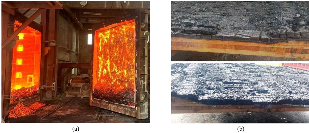
Fig. 9. Changes in the furnace (a) and in the residual char depth (b) due to heat delamination in CLT. CLT: cross-laminated timber.
