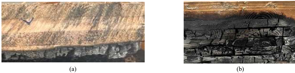
Fig. 10. Comparison of char layer formation according to adhesive of PUR (a) and PRF (b). PUR: polyurethane resin adhesive, PRF: phenol-resorcinol-formaldehyde resin adhesive.
