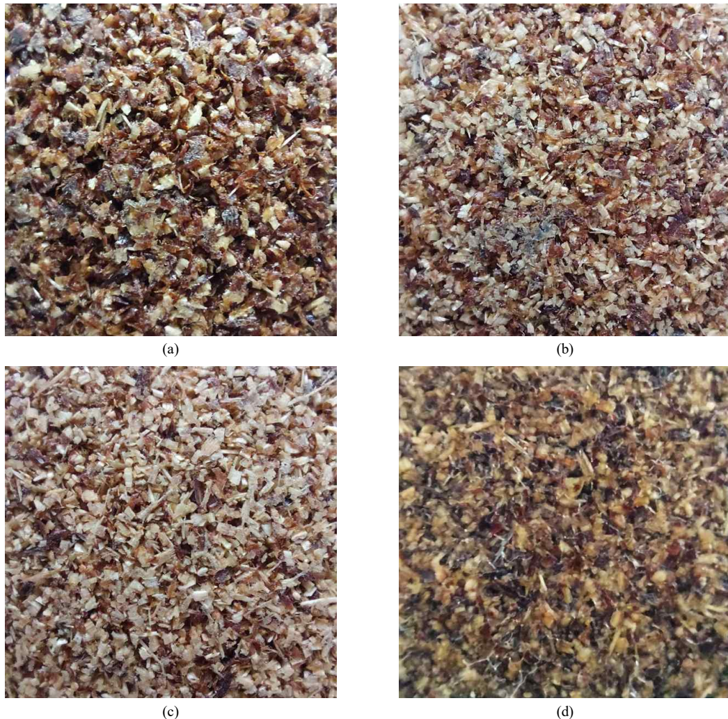
Fig. 1. Morphological appearance of ulin-sengon wood flour mixtures under different blending ratios and alkali treatment conditions. (a) 75% ulin:25% sengon, (b) 50% ulin:50% sengon, (c) 25% ulin:75% sengon, (d) 50% ulin:50% sengon.
