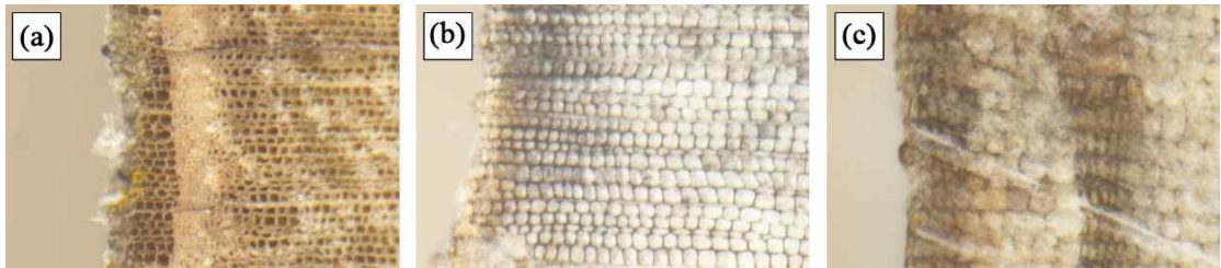
Fig. 3. Transverse thin sections of the Korean red pines that died in different seasons. (a) The outmost annual rings with earlywood, (b) not completed latewood formation, and (c) completed latewood formation.
