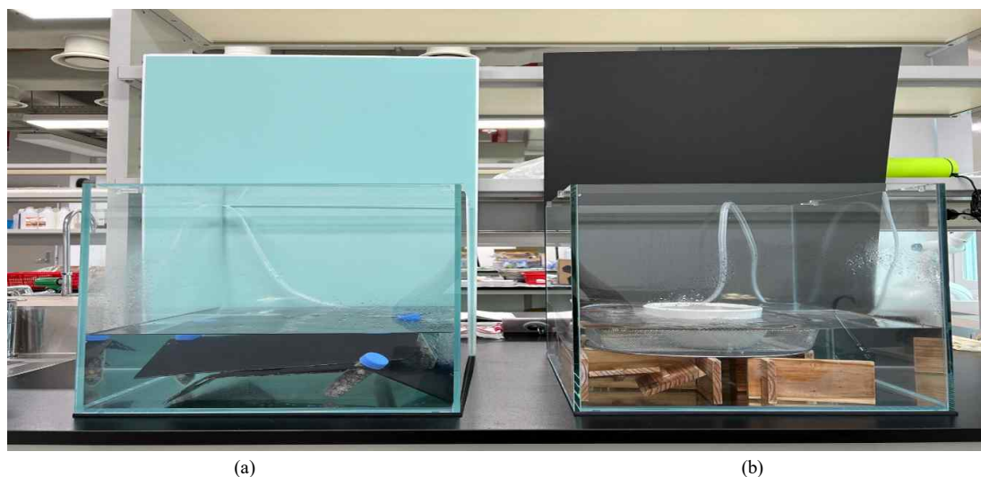
Fig. 3. Image showing how the quantities of microplastics generated from (a) plastic and (b) wooden shelters were compared, with both shelters immersed in the saline water in the glass aquarium.
