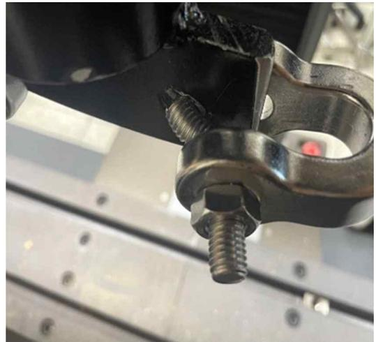
**Fig. 6.** Turnbuckle fixing bolt bending failure of A-2-a.
