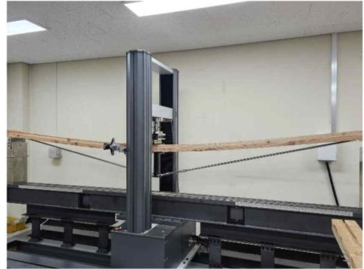
**Fig. 4.** Bending test progress.
