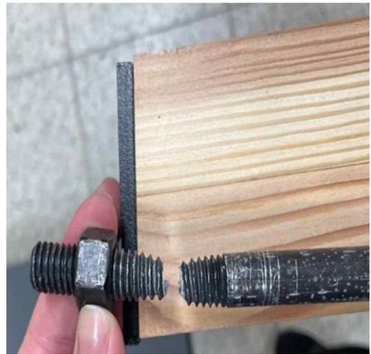
Fig. 8. Screw thread failure of A-1-a.
