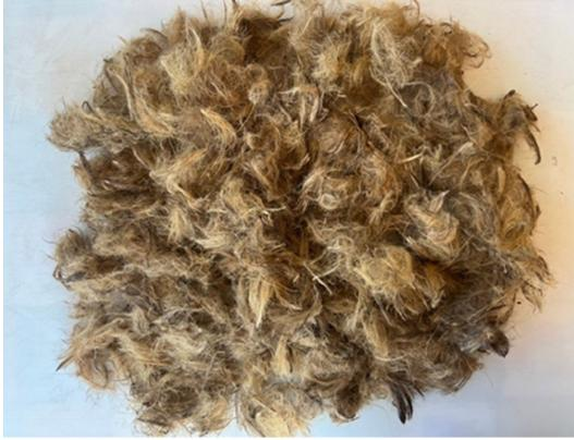
**Fig. 1.** Fiber from areca nut shells.
