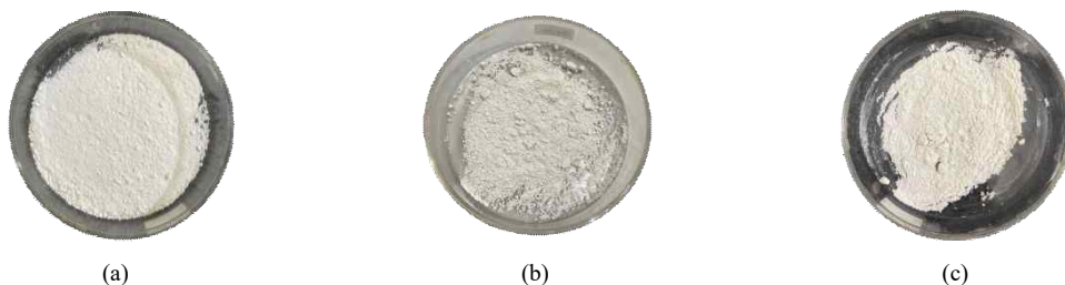
Fig. 4. Nanoparticle powder. (a) SiO 2 NP, (b) BN NP, (c) SiO 2 /BN NCP. NP: nanoparticles, BN: boron nitride, NCP: nanocomposite.
