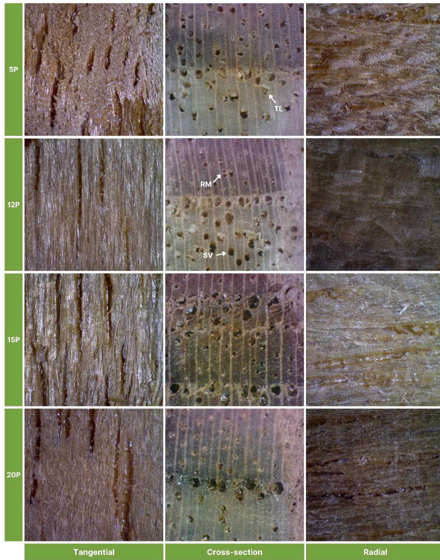
Fig. 3. Microscopic images ( 2.5 \times magnification) of tangential, cross-sectional, and radial sections of JPP (P) at ages 5, 12, 15, and 20. TL: tylosis, RM: radial multiples, SV: solitary vessel, JPP: Jati Plus Perhutani.
