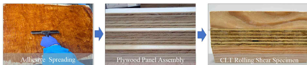
Fig. 1. Manufacturing process of plywood and CLT. CLT: cross-laminated timber.
