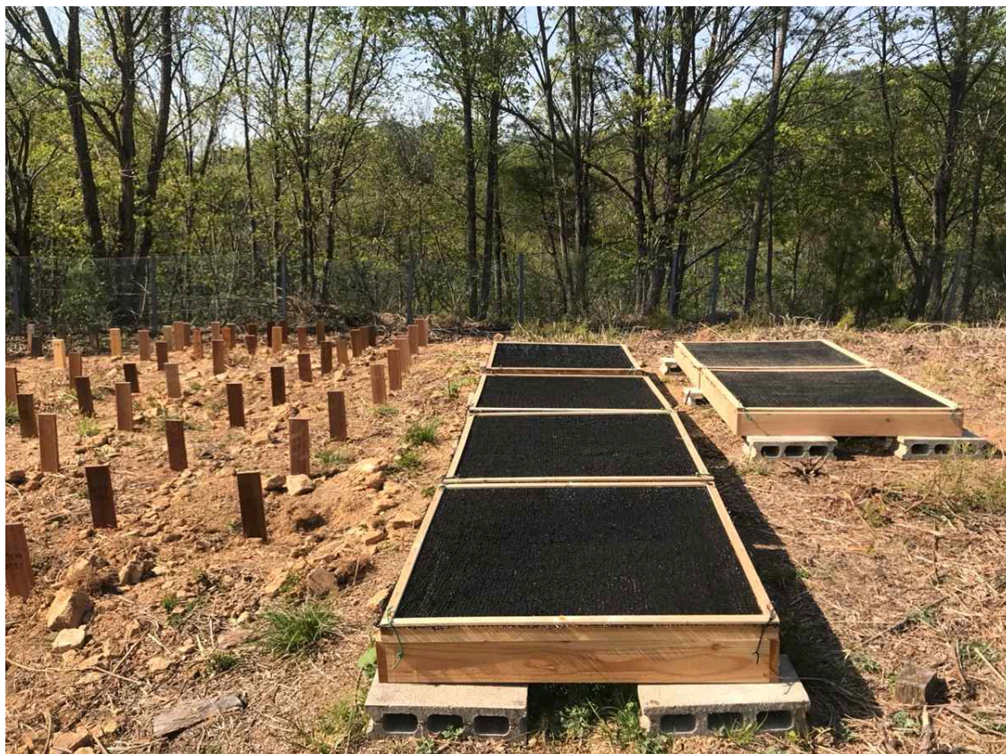
Fig. 1. Ground-proximity and stake tests at the outdoor exposure site.
